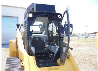
Supertrak is proud to offer an Industry Leading ½" Lexan® Front Door Kit for your Caterpillar® C-Series Models. The ½" Front Door Kit provides extra operator protection in operating environments such as applications like Forestry, Grading, or Recycling.
